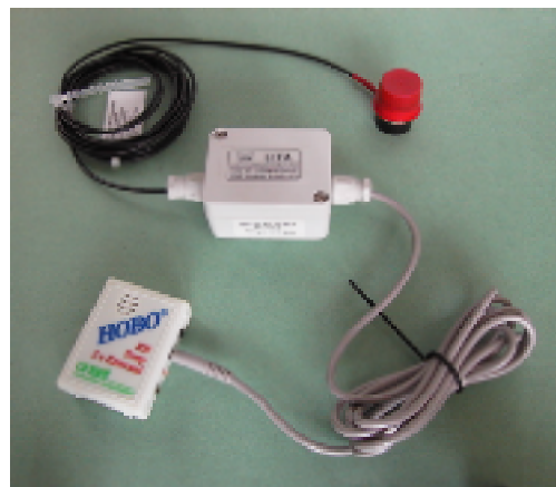
Figure 7: UTA to HOBO connection - A UTA serves as a link between a LI-COR sensor and the Onset HOBO data logger. The UTA amplifies the tiny current signal from the LI-COR sensor and outputs a voltage compatible with the HOBO.
