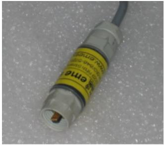
The SHT75PG above is mounted on a length of 3/8" PVC pipe, drilled 7/16" at both ends and tapped PG7. Connection is made to a cable. This unit is shown with the protective cap removed for fastest response. A level of protection appropriate to the environment can be installed. Observe that the open PG7 guards the sensor from breakage, but allows for good air flow.
