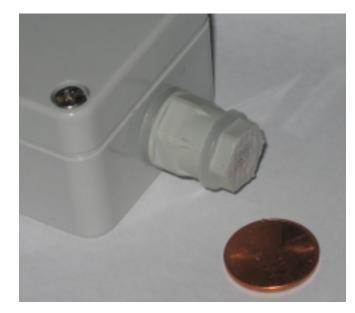
The SHT75PG here is mounted on a sealed polycarbonate enclosure. The sensor element itself is protected under a membrane permeable to water vapor. The enclosure can be drilled 7/16" and tapped PG7, or the enclosure can be drilled 1/2" and a PG7 nut (included) installed on the inside. Inside the enclosure can be a data logger or transition wiring to a cable.
