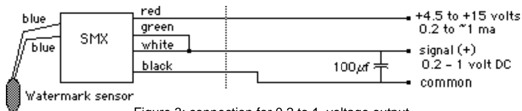
Figure 3: connection for 0.2 to 1 voltage output
