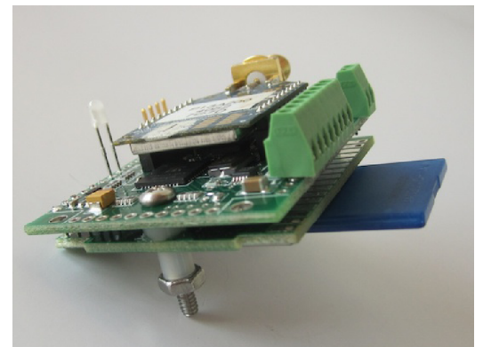
Core module in sandwich, with SD card below and XBee in socket, and terminals for thermocouples.
