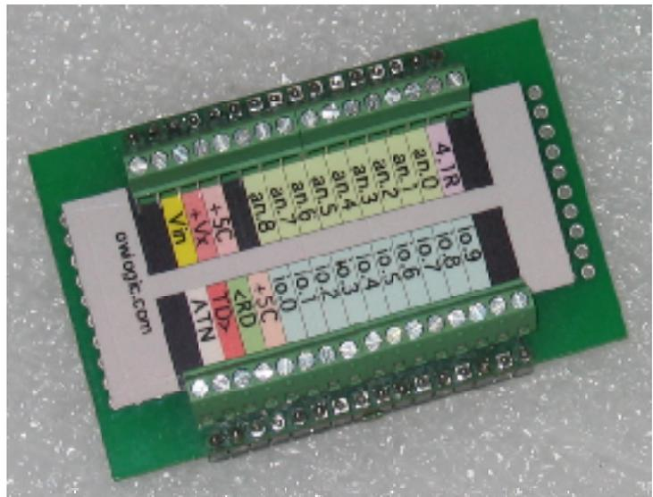
has mounting holes for #4-40 screws, aligned with the mounting holes in the OWL2pe module.
