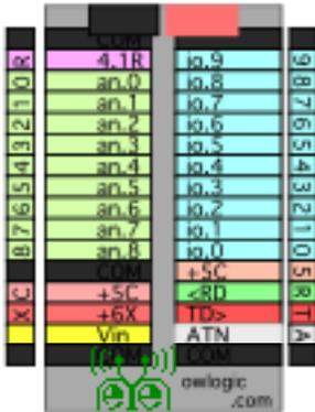
Input power from 5.5 to 15 volts DC comes in on the terminal "Vin". The operating current is up to 17 milliamps to operate the OWL itself, plus whatever current is required by external circuitry. In sleep mode, the current consumption drops to less than 100 microamps.
