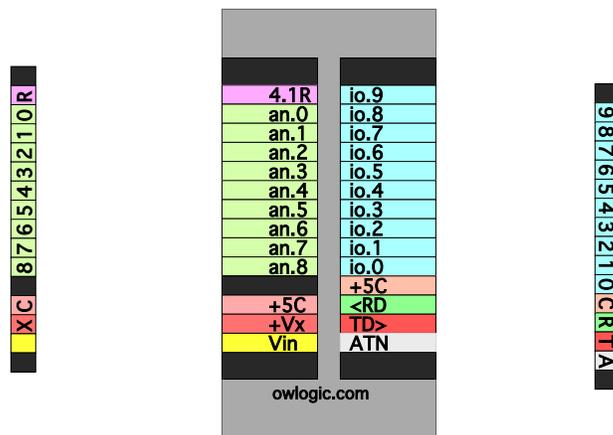
This diagram can help to plan and document sensor wiring to the top board TB11032
