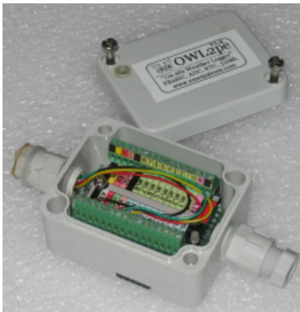
An OWL2pe and a TB11032, trimmed to fit in a small polycarbonate enclosure. Includes an external LED indicator and an socket header for data offload.
