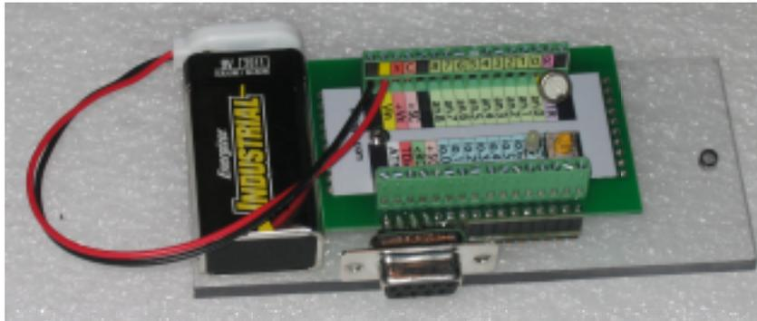
A TB11032 and OWL2pe, set up as a demo. It is mounted on a polycarbonate plate, and the demo setup includes a battery, a DB9S connector, an led, and a potentiometer as analog input and a switch as digital input.
