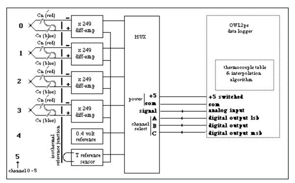
For biological applications, we recommend type T thermocouples, which have the lowest margin of error (due to the attainable purity of the metals copper and constantan), and perform well in either mildly reducing or mildly oxidizing situations and at moderate temperatures -200 to +350 °C. Type K thermocouples are also popular for general purpose applications and a wider temperature range up to -200 to +1350 °C
